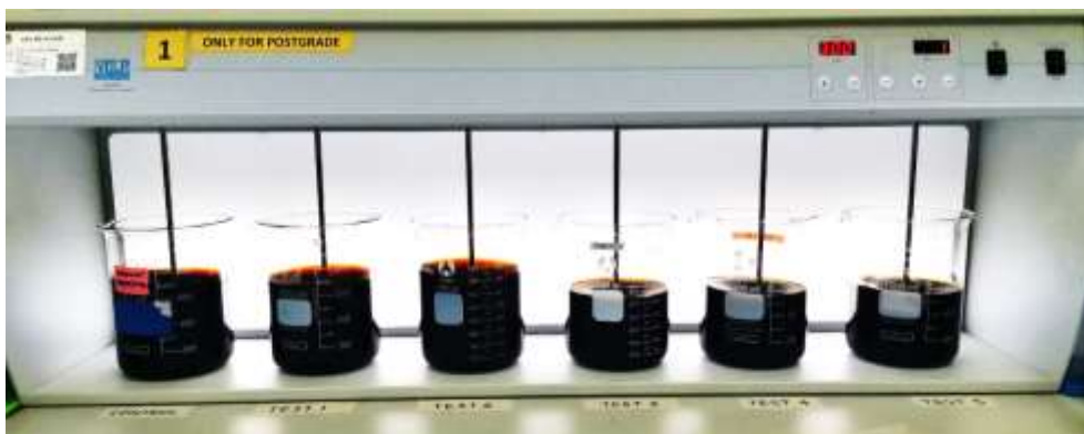
Figure 1. The setup of the jar test
