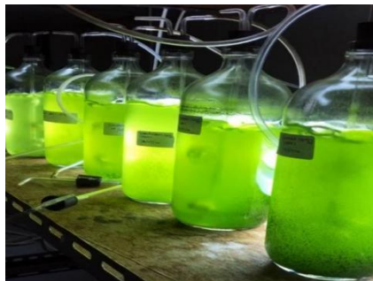
Figure 3. Cultivation of microalgae inoculums in 1 L glass bottles
