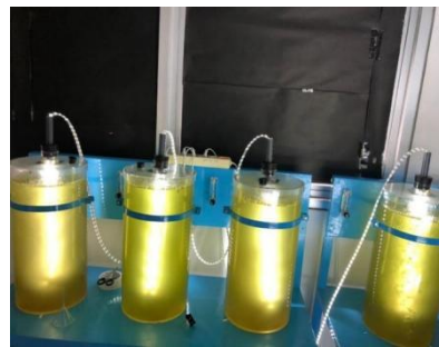
Figure 6. Cultivation of microalgae on ADDMW medium
